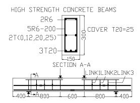
Fig 2. Reinforcement details and position of strain gauges for the High Strength Concrete test specimen
