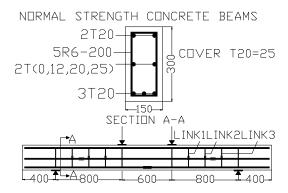
Fig 1. Reinforcement details and position of strain gauges for the Normal Strength Concrete test specimen
