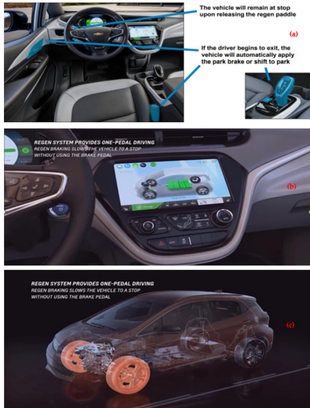
Figure 1. Image showing the regenerative braking system for one-pedal driving for an electric vehicle. It is designed with a display showing simplified mechanisms on the pedal braking, battery savings and the energy efficiency indicator. (a) Interior of the EV with the one-pedal driving and gear system, (b) Regen braking system for the EV with display system, and (c) visualization of the EV's regen system which provides one-pedal driving (Courtesy: General Motors).
