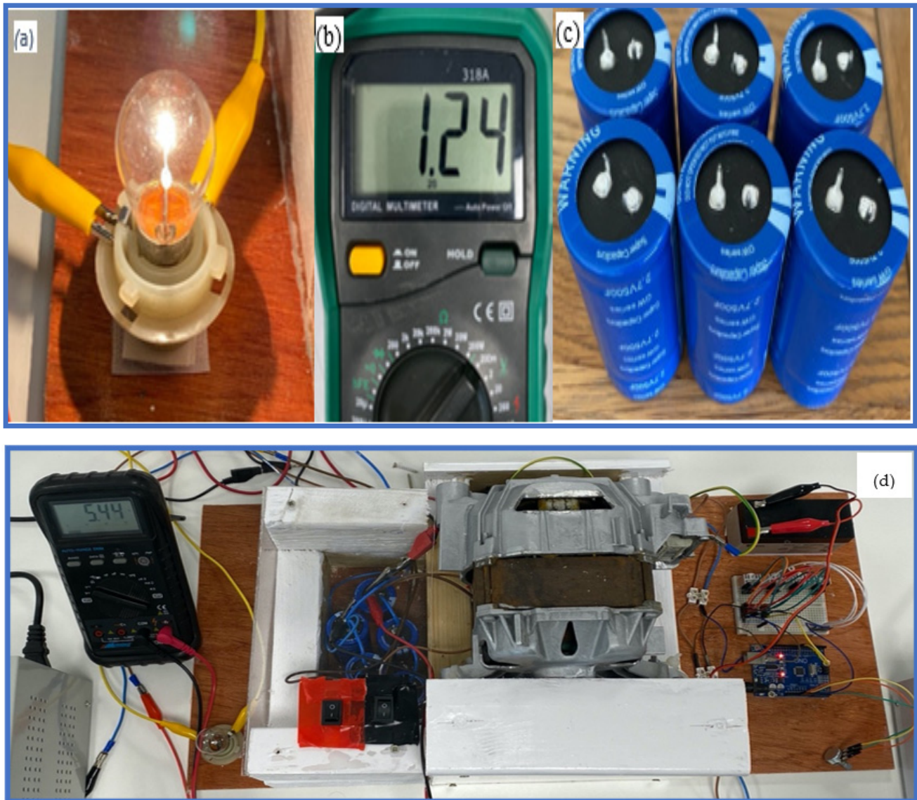
Figure 13. Experimental resources: (a) a 12 V 22 W bulb load, (b) a 12 V bulb's current rated using a meter, (c) a supercapacitor bank and (d) the experimental setup showing the red switch, black switch, DC motor, light bulb, Multimeter, testing terminals, connection cables and the circuit board.
