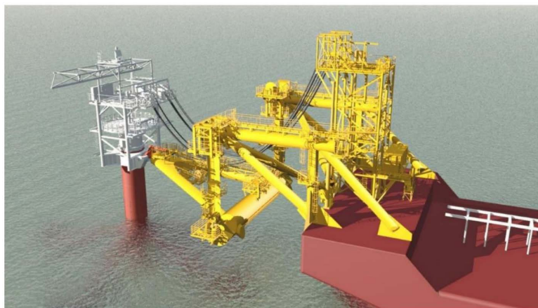
Figure 7—FPSO/FSRU Moored by Soft Yoke Mooring Systems (SYMS)
