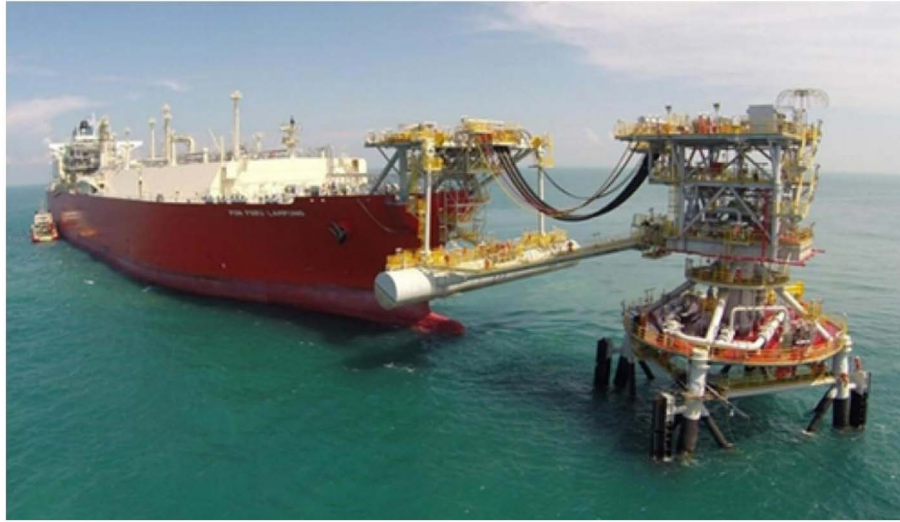
Figure 6—FPSO/FSRU Moored by Tower Yoke Mooring (TYM)
