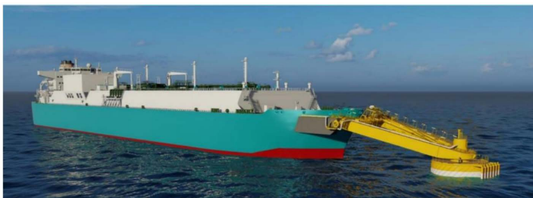
Figure 8—FPSO/FSRU Moored by Catenary Anchor Leg Rigid Arm Mooring (CALRAM)
