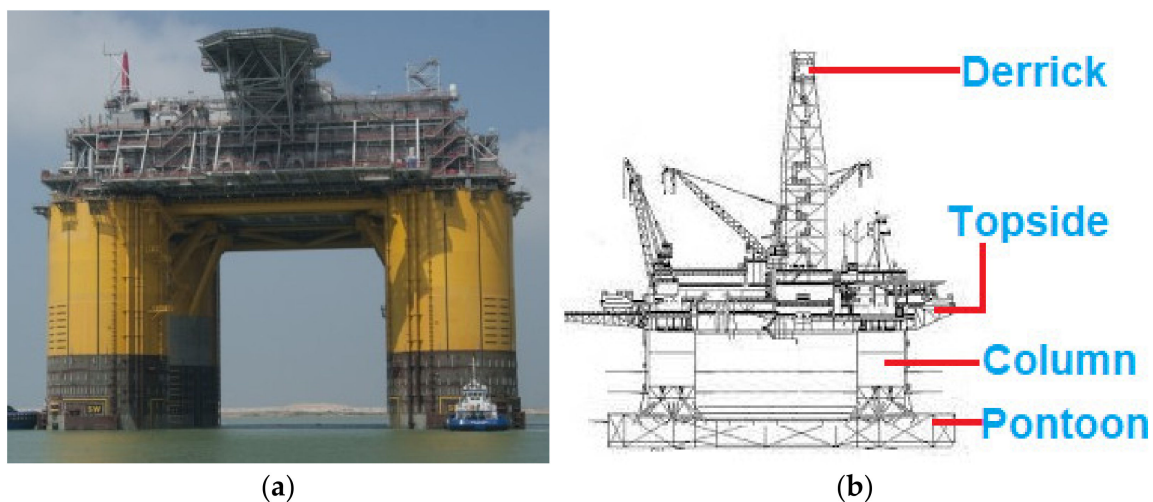
Figure 10. Semisubmersibles showing (a) Appomattox Semi-Submersible oil platform in GoM installed in 2019 (Courtesy: Shell), and (b) an illustration of part of a semisubmersible.
