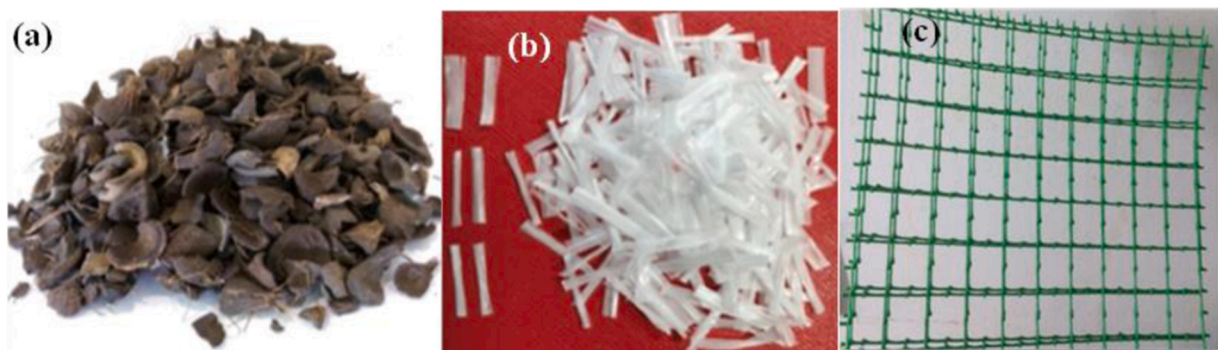
Fig. 1. (a) Oil palm shell lightweight aggregates (b) Fibrillated polypropylene fibre (c) Extruded polypropylene mesh.
