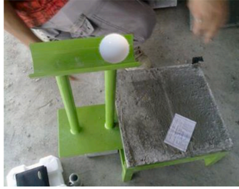
Fig. 5. Illustration of impact test arrangement using impact test rig.
