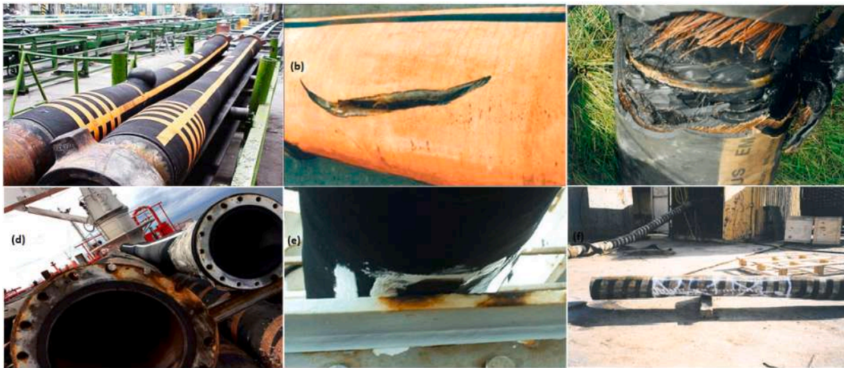
Fig. 25. Collage of different hose failure modes, showing (a) pressure test with leaking liner, (b) floating hose after a propeller cut, (c) excess cover damage down to breaker fabric, (d) corrosion and heavy wear of the hose flange that had a service life of 14 years, (e) hose damage from abrasion cut on cover (f) crushed 16 inches submarine hoses after excessive load landed on it, (Courtesy: PSI, 4Subsea, Continental Dunlop & Trelleborg).
