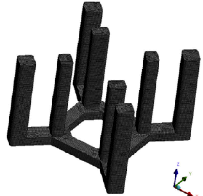
Fig. 7. Hydrodynamic panel model of the PC semi (in ANSYS AQWA R2 2020).
