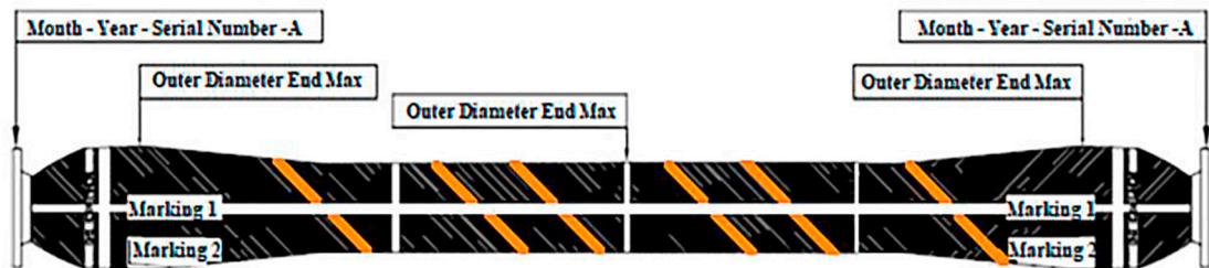
Fig. 7. Marine hose segment of 12m in length depicting markings with descriptions.
