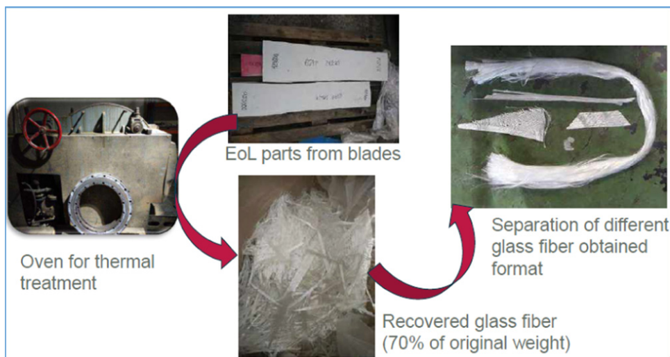
Fig. 19 Thermal recycling for wind turbine blades. Courtesy: FiberEUse. Source: Garcia, S., Arcarazo, A., 2019. Large scale demonstration of new circular economy value-chains based on the reuse of end-of-life fiber reinforced composites. In the proceeding WindEurope Conference & Exhibition, pp. 1–12. 2–4 April 2019, Workshop on blade disposal. Bilbao: FiberEUse.
