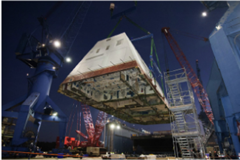
Fig. 26 The 1000-t deckhouse of destroyer USS Zumwalt (DDG 1000) is craned toward the deck of the ship at General Dynamics Bath Iron Works. The deckhouse is primarily made from balsa-cored carbon fiber using vacuum assisted resin transfer molding. Reproduced from Job, S., 2015. Why not composites in ships? Reinforced Plastics 59 (2), 90–93. doi:10.1016/j.repl.2014.12.047.
