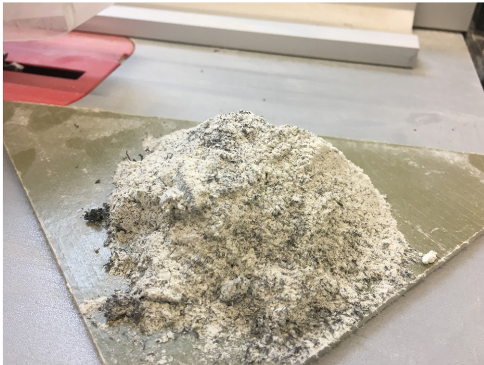
Fig. 5 Glass fiber dust waste from Strongwell's Extren laminated glass fiber composite sheet.
