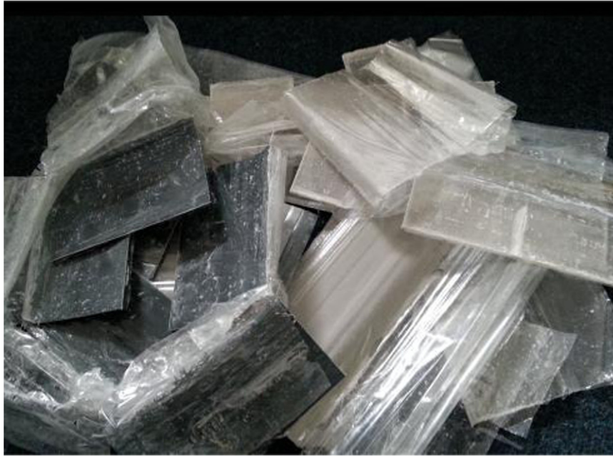
Fig. 4 Glass reinforced polymer trimmed waste. Courtesy: Filon products.
