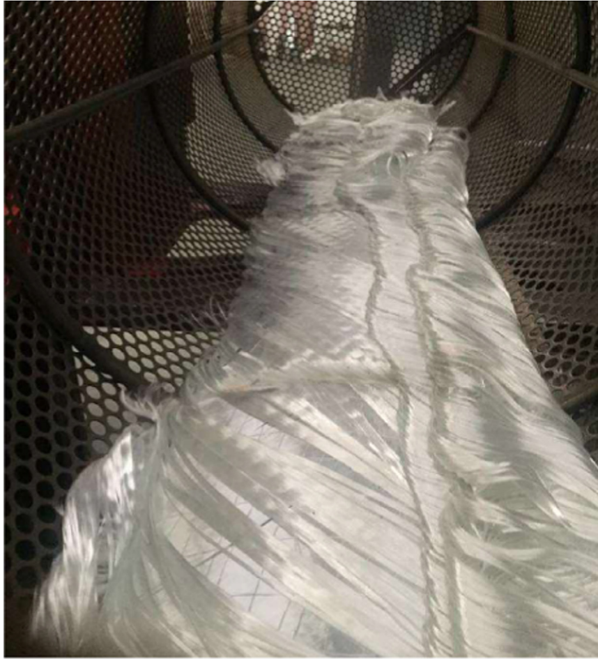
Fig. 23 The result from recycling a wind blade made of glass fiber. Courtesy: Reciclaia.
