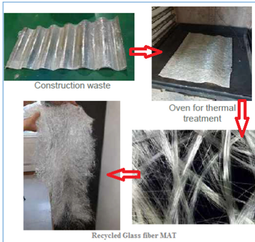
Fig. 20 Thermal recycling of aeronautic waste. Courtesy: FiberEUse. Source: Garcia, S., Arcarazo, A., 2019. Large scale demonstration of new circular economy value-chains based on the reuse of end-of-life fiber reinforced composites. In the proceeding WindEurope Conference & Exhibition, pp. 1–12. 2-4 April 2019, Workshop on blade disposal. Bilbao: FiberEUse.
