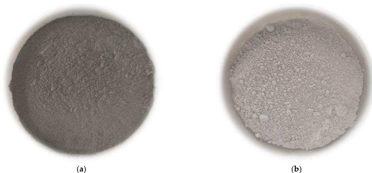
**Figure 1.** Morphology of fly ash and slag used in the test. (a) Fly ash; (b) Slag.
