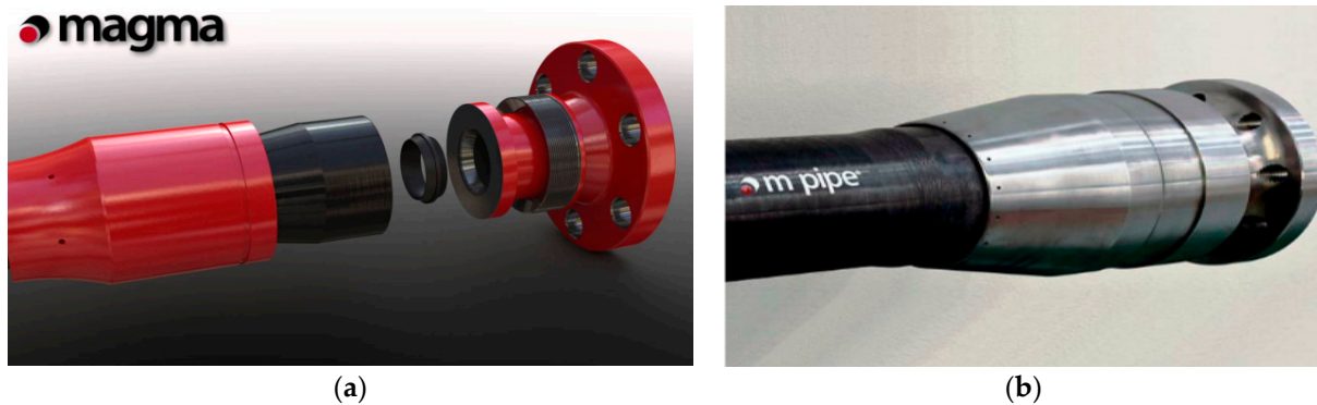
Figure 1. Composite riser pipe section with Magma m-pipe end fittings, showing (a) end-fitting with fittings, pipe, seal and smaller flange (b) end-fitting coupled with pipe and bigger flange with unique bolt ends (courtesy: Technip FMC’s Magma Global).
