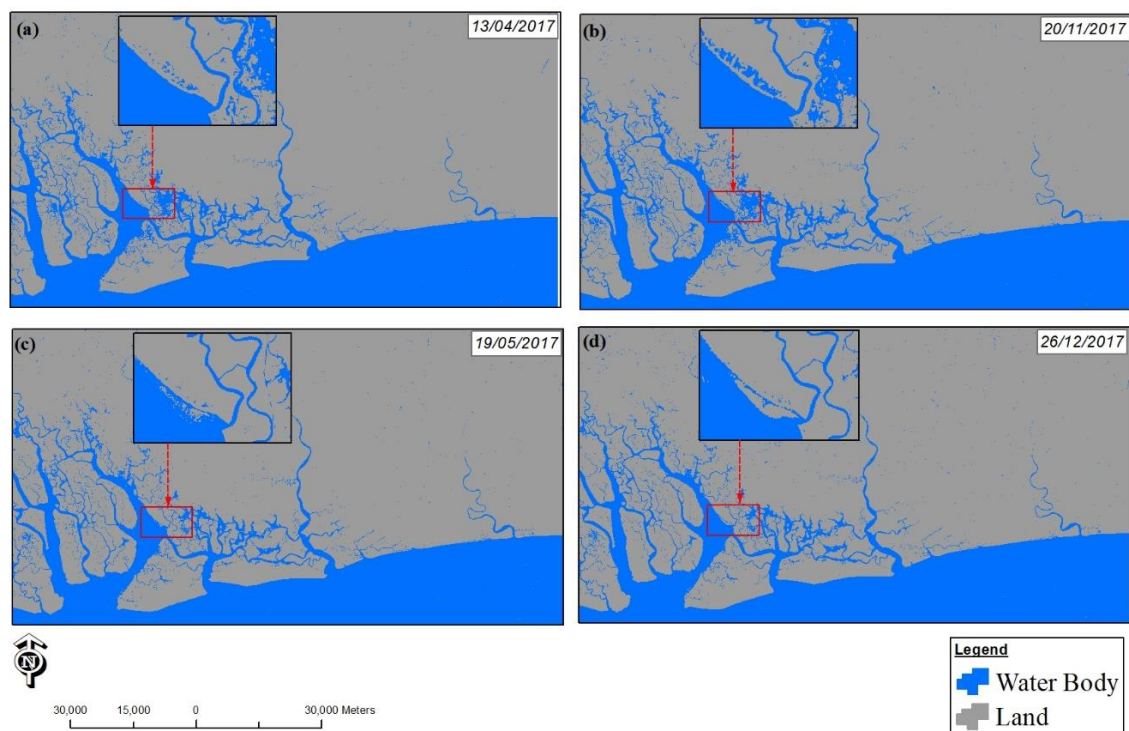
Figure 8. Binary classification of Sentinel-1 images into land and water body classes, showing the images retrieved on (a) 13 April 2017, (b) 20 November 2017, (c) 19 May 2017, and (d) 26 December 2017.
