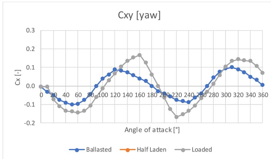
Fig. C1. Current coefficients along surge direction for Suezmax.
