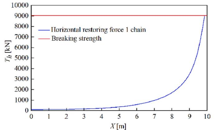
**Fig. 3.** Horizontal restoring force in one chain due to the horizontal displacement buoy in line with chain.
