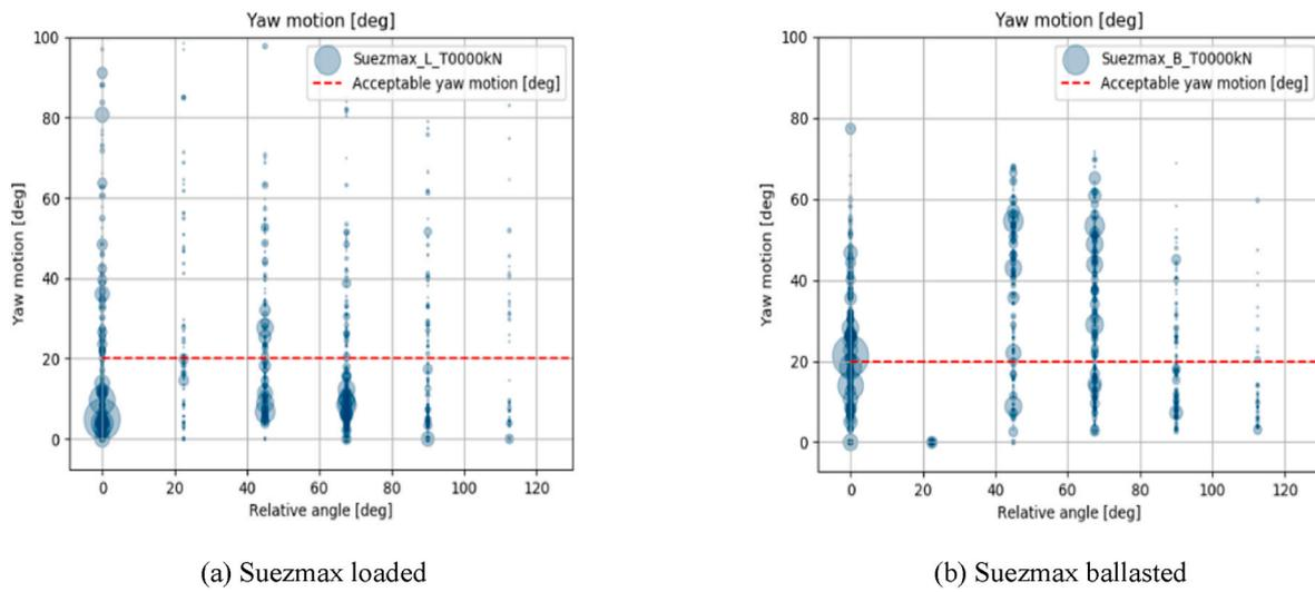
Fig. 11. Effect of the relative angle between wind and current direction on the yaw motion for Suezmax in case no pullback force is applied.
