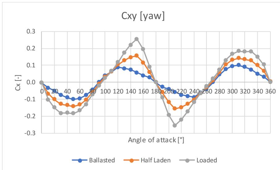
Fig. B1. Current coefficients along surge direction for VLCC.
