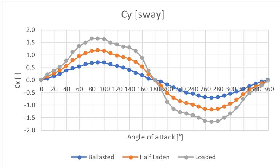
Fig. A3. Wind coefficients along yaw direction for both tankers -VLCC and Suezmax.
