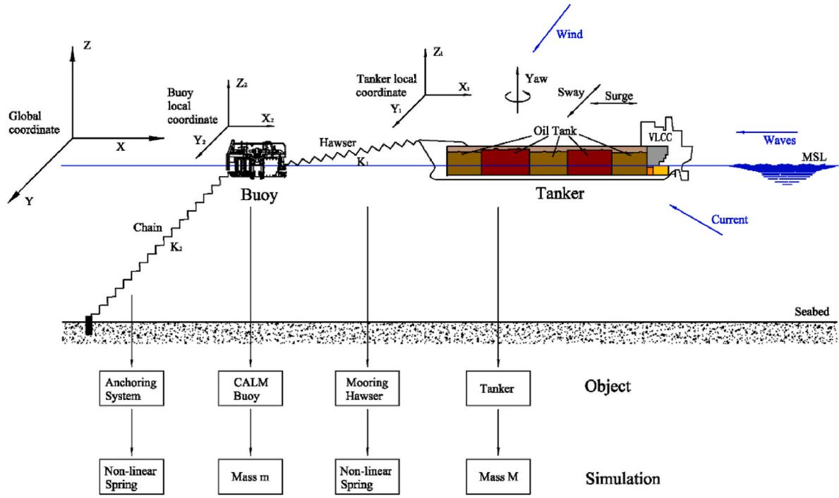
Fig. 2. Dual-spring hydrodynamic response model of the CALM moored tanker system.
