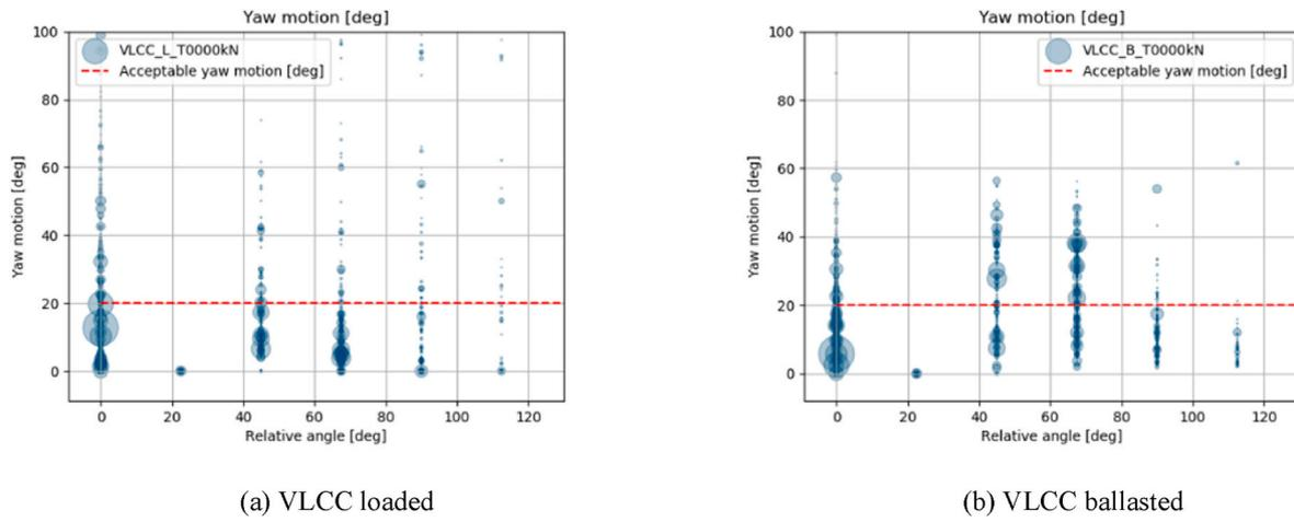
Fig. 10. Effect of the relative angle between wind and current direction on the yaw motion of the VLCC in case no pullback force is applied.
