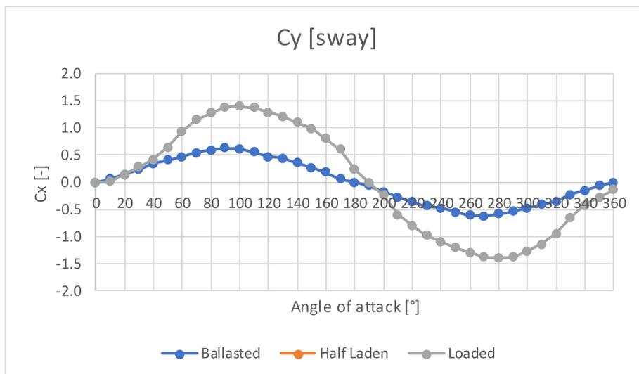
Fig. B3. Current coefficients along yaw direction for VLCC.
