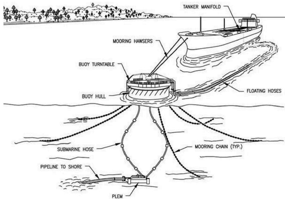
Fig. 1. Schematic of a typical catenary anchor leg mooring (CALM) system (Shell DEP 37, 2011). Permission was obtained to adapt, reuse and reproduce as it was published in an open access publication. Publisher: Hindawi; Copyright year: 2022; Secondary Source: Ju et al., 2022a).
