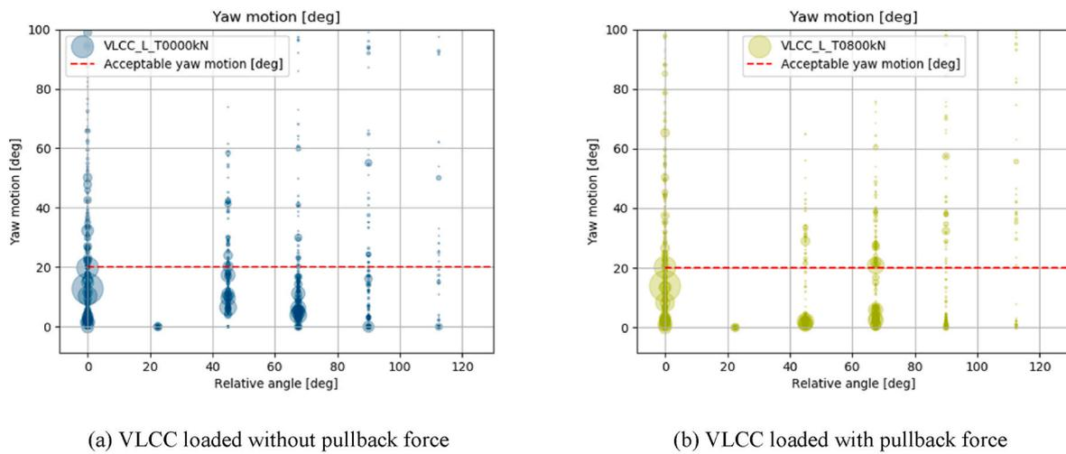
Fig. 12. Effect pullback force on yaw motion for VLCC loaded.
