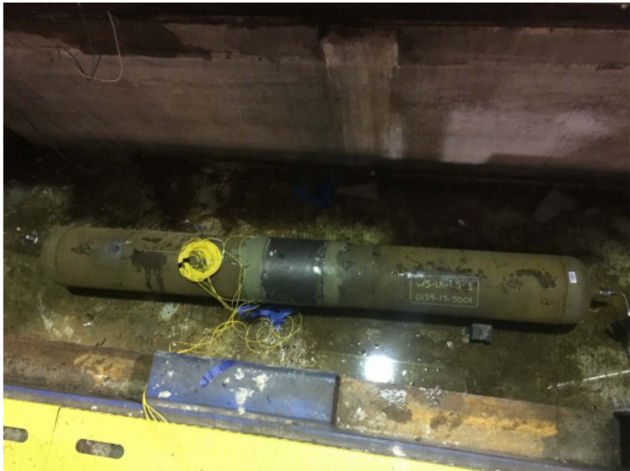
Figure 16. Typical composite pipe repaired with ComposiSleeve™ sample (Reprinted/adapted with permission from Dr. Chris Alexander; Source: Ref. [63]. Copyright year: 2018, copyright owner's name: ASME & Dr. Chris Alexander).
