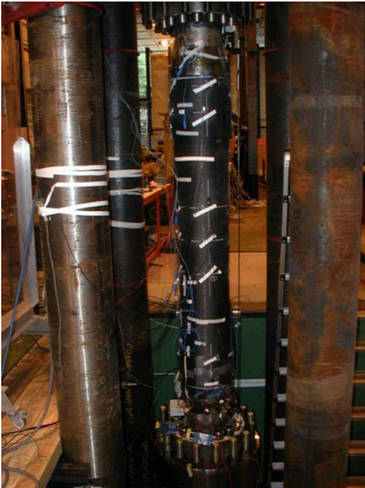
Figure 3. A fatigue testing rig for composite marine riser showing sensors, cables, and other monitoring devices used (Reprinted/adapted with permission from Ref. [109]. Copyright year: 2014, copyright owner's name: Prof. Andreas Echtermeyer, NTNU).
