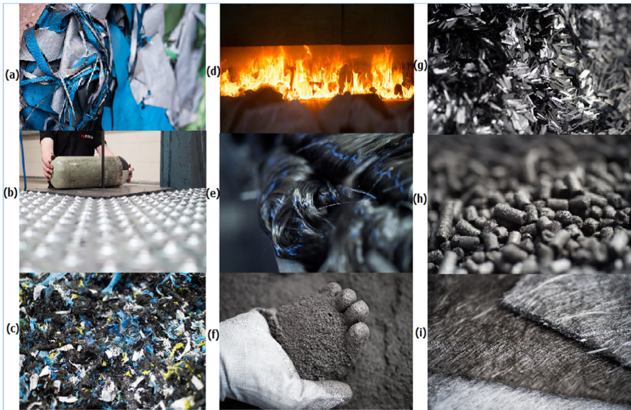
Fig. 10 Steps (a)–(i) involved in the carbon fiber recycling process. Courtesy: ELG Carbon Fibre, 2017. Why Recycle Steel? Coseley, West Midlands, UK. Available at: https://www.recycle-more.co.uk/why-recycle/why-recycle-steel- .
